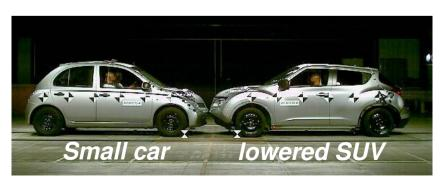
Test 2: Adjusted height (height of front rails of SUV was aligned with that of small car)
