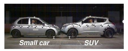
Test 1: Original height (front rails of SUV were higher than that of small car)
