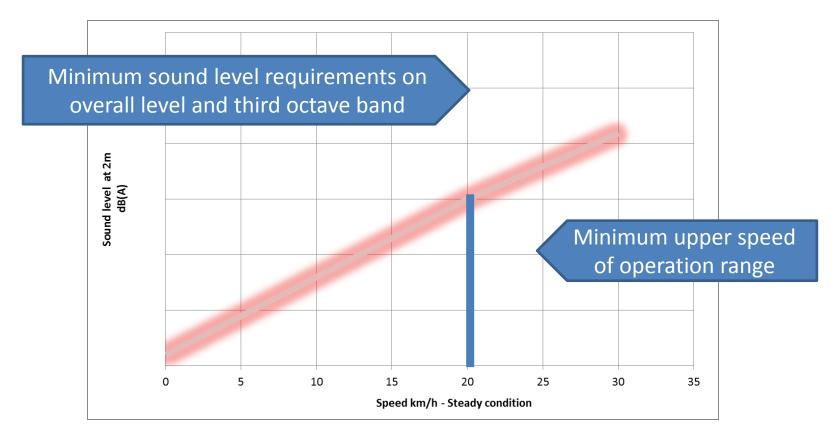
For vehicle equipped with AVAS in activation the difference between the minimum sound vehicle (overall level) and the red curve shall be less than xx dB.
