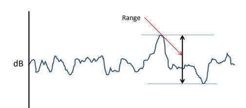
9.7.6 Reporting and use of background noise for analysis in 1/3 octave bands. The background, or ambient noise, shall be measured for duration of at least 20-seconds before and after a series of vehicle tests. The measurements shall be made with the same microphones and microphone locations used during the test.
