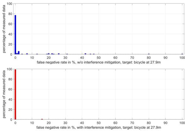
Fig. 6. Laboratory measurements: false negative for a bicycle target at 27.9m, upper figure: without interference mitigation, lower figure: with uncooperative interference mitigation.
