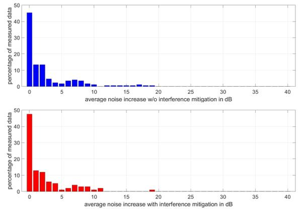
Fig. 4. Laboratory measurements: average increase of noise level due to interference, upper figure: without interference mitigation, lower figure: with uncooperative interference mitigation.
