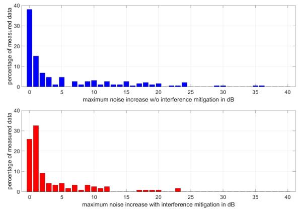
Fig. 5. Laboratory measurements: maximal increase of noise level due to interference, upper figure: without interference mitigation, lower figure: with uncooperative interference mitigation.
