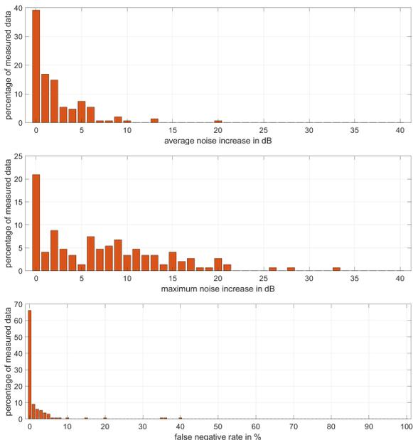
Fig. 7. Boxberg measurements: scenario UV-1, upper figure: average increase of noise level due to interference, middle figure: maximum increase of noise level due to interference, lower figure: false negative.
