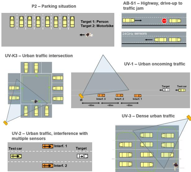
Fig. 3. Examples for test scenarios measured on Boxberg Proving Grounds.
