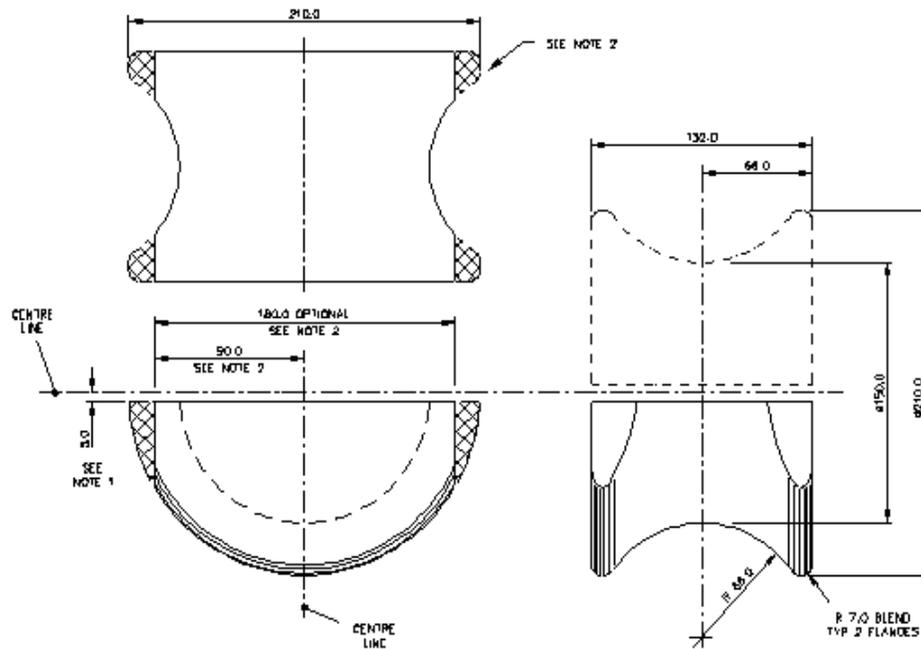
Figure 23: Details of dynamic lower legform certification impactor face
