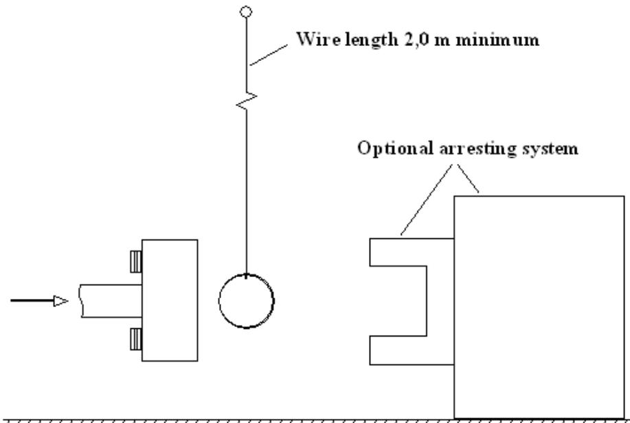
Figure 24. Test set-up for dynamic upper legform impactor certification test
