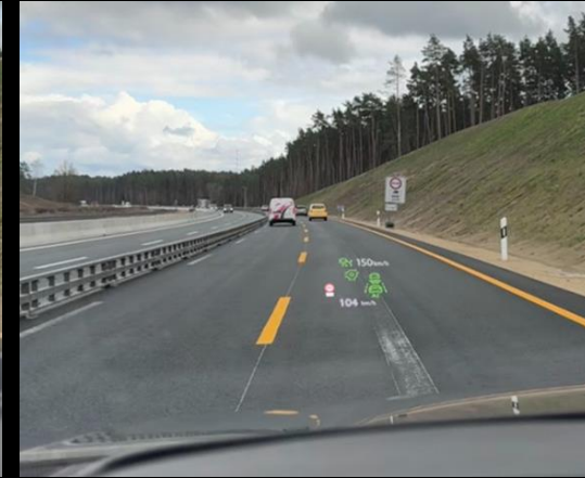
Photo of standard FVA content speed sign size reduced to a size as if it would have to fulfill a 35% requirement of JAMA basic figure
