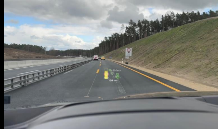
Photo of standard FVA content speed sign digitally overlaid with 75% height of JAMA basic figure and 100% outline of basic figure
