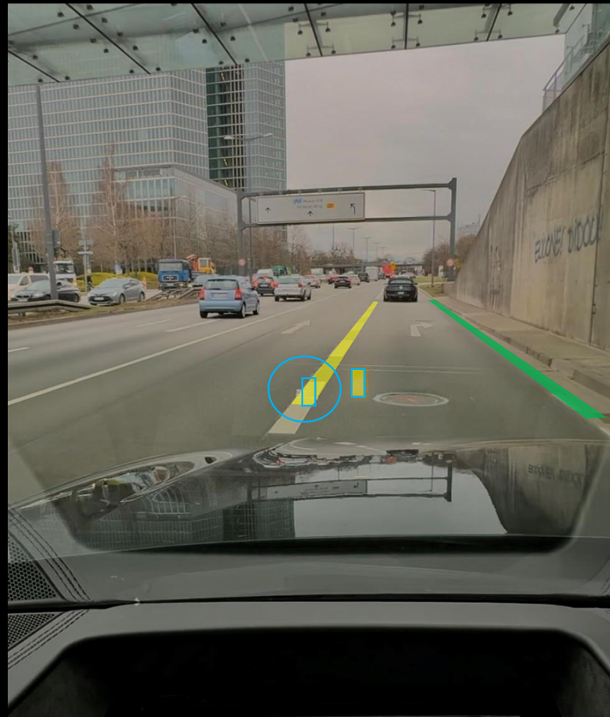
Example: lane departure warning (digitally added) vs. size 75% of JAMA basic figure size
