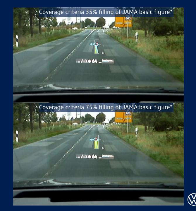
Comparison of navigation advance notice size vs. 35% and 75% of JAMA basic figure filling
