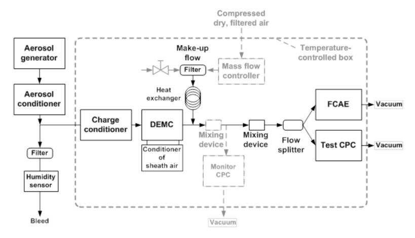
The calibration setup with FCAE as reference instrument. Dashed lines in grey show equipment that is not required, but highly recommended.
