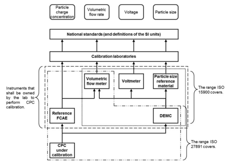
The four directly traceable quantities do not completely underpin the quantity measured by the CPC – particle number concentration. The extra parameter - the mean charge per particle used for the calibration - is determined by the experimental setup, and is controlled by the procedures and checks described in Annex D of ISO 27891.
