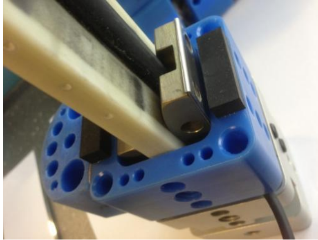
Figure 26 . Fitting thin bone spacer with captive shim
