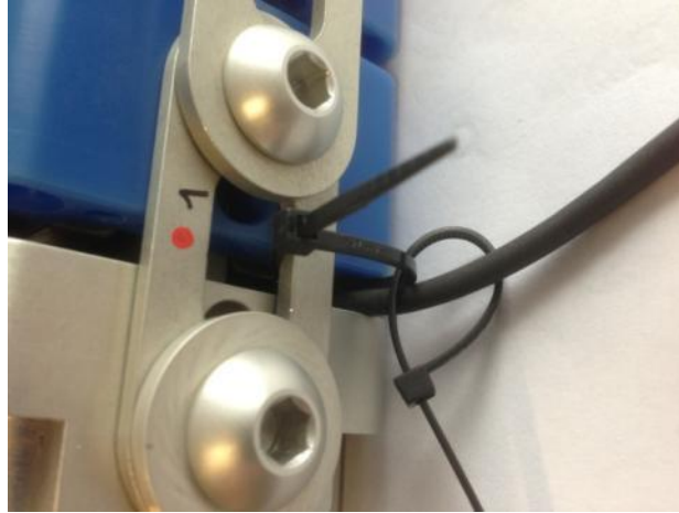
Figure 27 . Bone exit cable restraint use cable ties (ties not shown trimmed or tightened)
