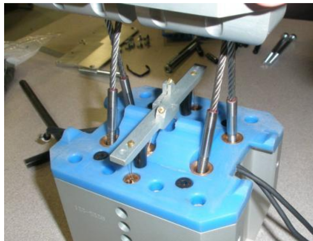
Figure 33 . Cross wire feed through on knee
