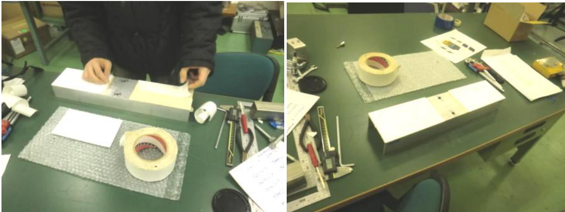
Figure 45 . Example of fixing PTFE sheet to base plate
