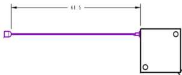
Figure 44 . String potentiometer pull wire length \pm 1mm
