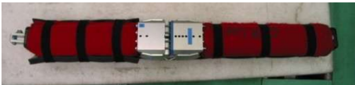
Figure 42 . Rubber flesh tied on with Velcro
