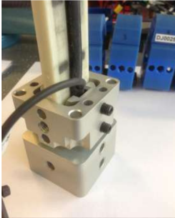
Figure 24 . 133-8129 base with 133-5514 segment, bone clamps and bone assembly
