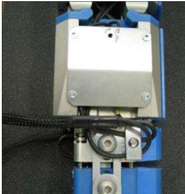
Figure 17 . Clamping Arrangement and Position for Off board Wires
