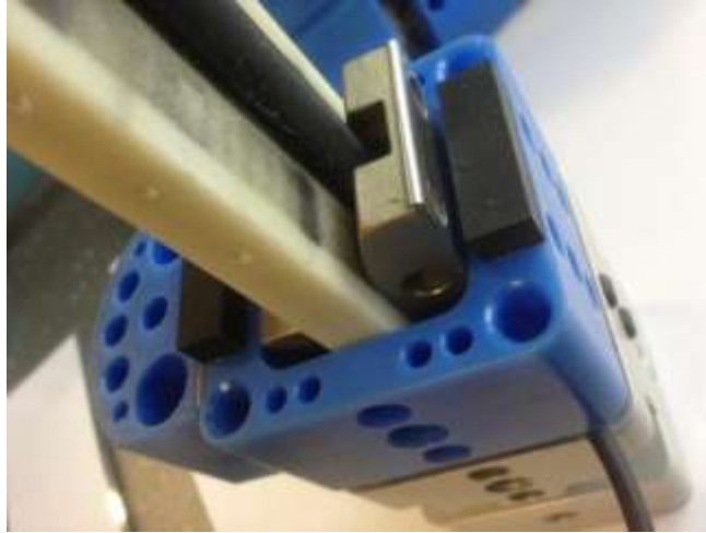
Figure 26 . Fitting thin bone spacer with captive shim
