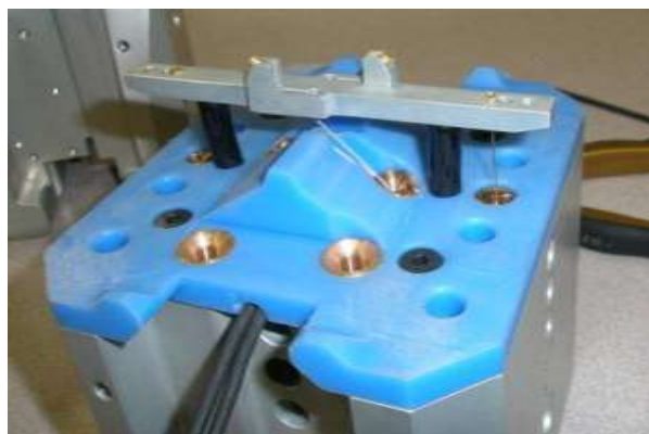
Figure 32 . Attachment plate, crimp wires in tension with spacers ready for knee femur block assembly
