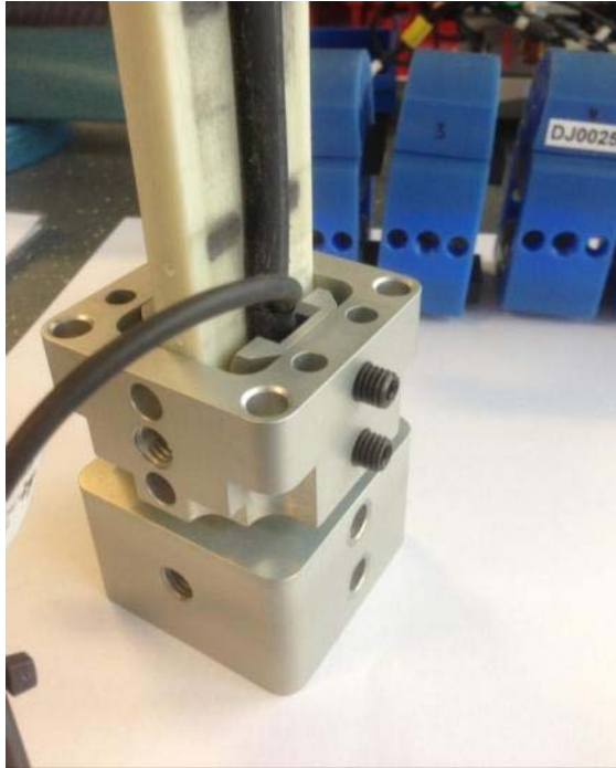
Figure 57 . 133-8129 base with 133-5514 segment, bone clamps and bone assembly
