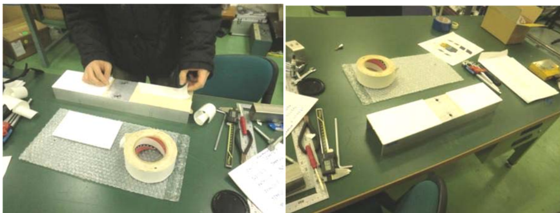
Figure 78 . Example of fixing Teflon sheet to base plate
