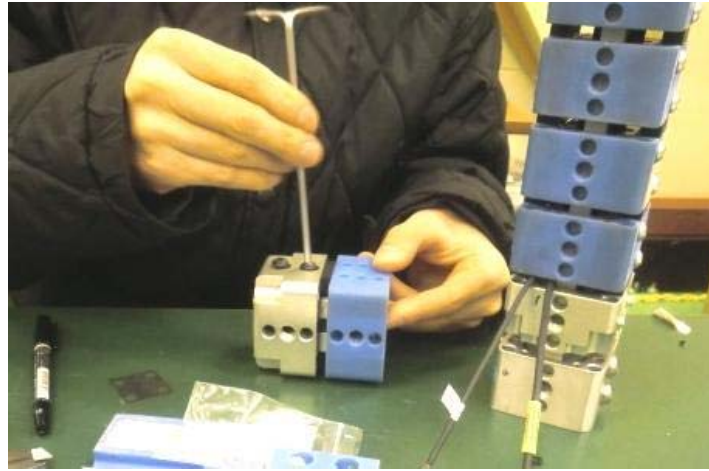
Figure 69 . Assembly of last two segments on tibia
