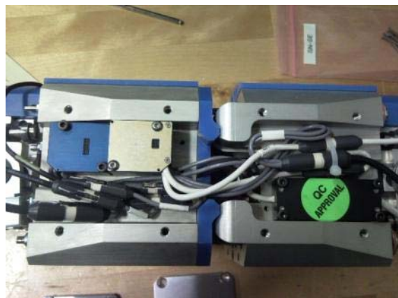
Figure 38 . Left side wiring example of 24 channel SLICE
