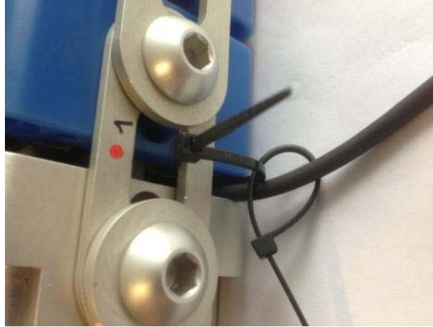
Figure 60 . Bone exit cable restraint use cable ties (ties not shown trimmed or tightened)
