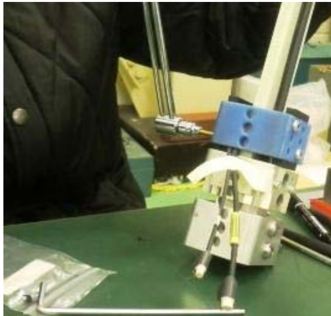
Figure 58 . Fitting and tightening first blue segment
