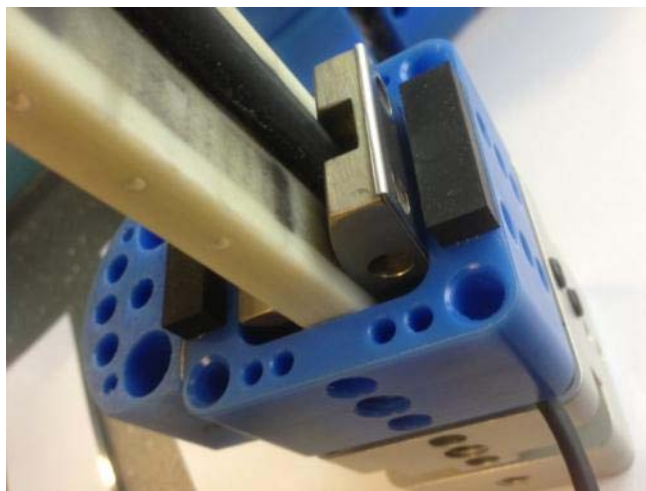
Figure 59 . Fitting thin bone spacer with captive shim
