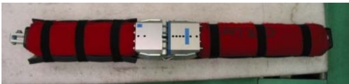
Figure 75 . Rubber flesh tied on with Velcro
