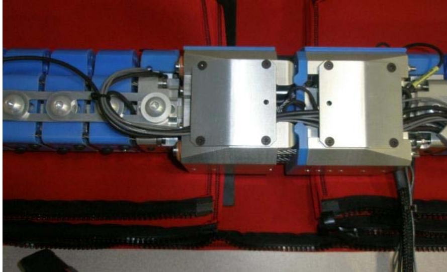
Figure 10 . Wire routing out of segment for optional sensors Detail A in upper knee
