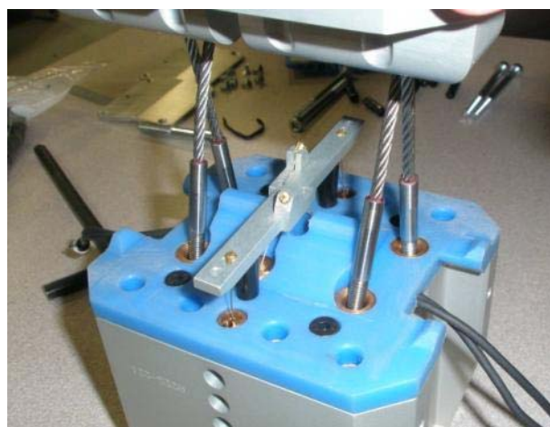
Figure 66 . Cross wire feed through on knee
