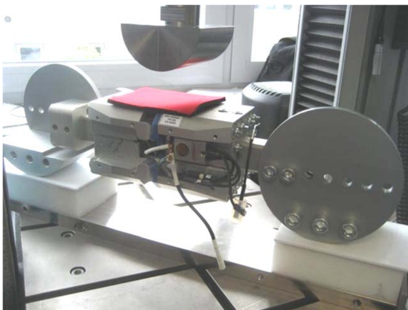
Figure 84 . Knee Certification Fixture
