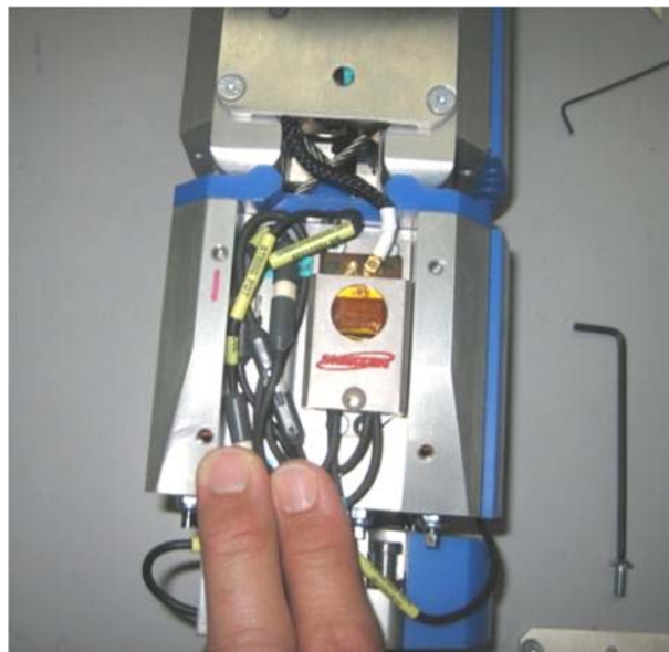
Figure 28 . Bottom right hand side of knee M=BUS 24 channels, sensors connected
