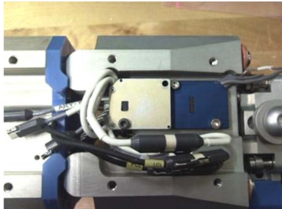
Figure 37 . Optional SLICE unit 24 channel option (right side)
