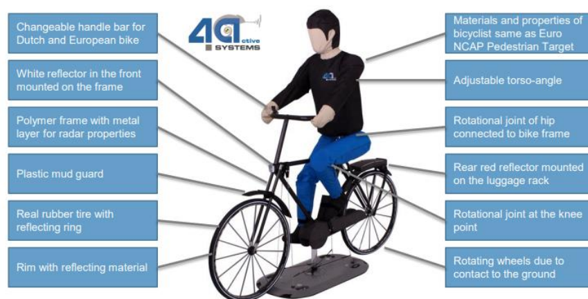
Figure 13 4a Cyclist dummy developed within the CATS project as presented at the FISITA in 2016
