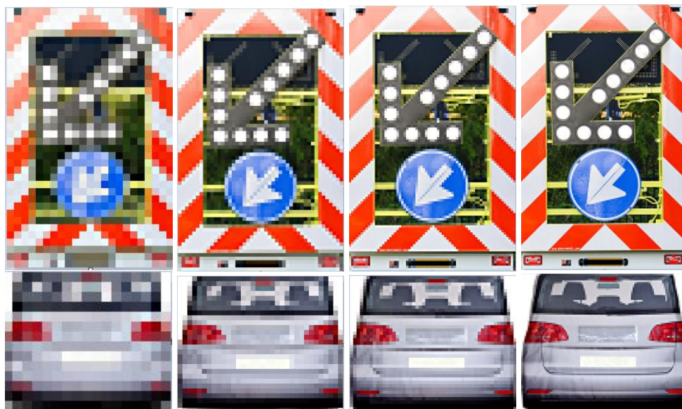
Figure 10 Image of a traffic arrow trailer (width 2.335m) and the EVT target (width 1.712m) at different pixels per meter (10, 20, 30 and 60 from left to right). The traffic arrow trailer corresponds to 23, 46, 70 and 140 and the EVT target corresponds to 17, 35, 51 and 103 pixels in width respectively
