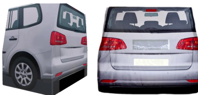
Figure 3 European Vehicle Target (EVT) which can be used in the approval process of AEB in trucks.
