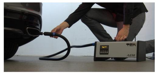
• Instrument : Particle counter with spec's according to NPTI-working group
