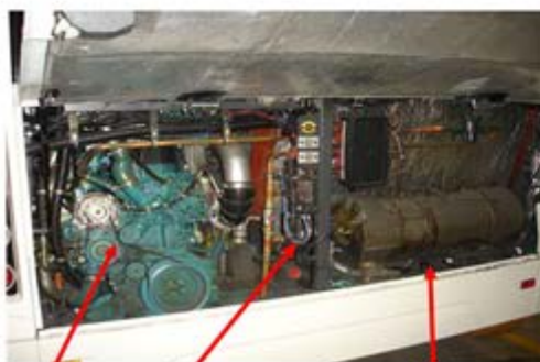
Engine SCR CRT Combustion engine and CRT + SCR -System
