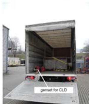
Vehicle H&I fitted for on-road measurements with NOx sensor, CLD and 3000 kg load.
