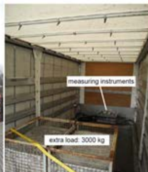
Vehicle H&I fitted for on-road measurements with NOx sensor, CLD and 3000 kg load.
