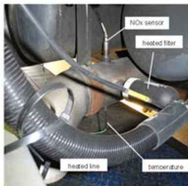
Vehicle exhaust tailpipe equipped for chassis dyno measurements
