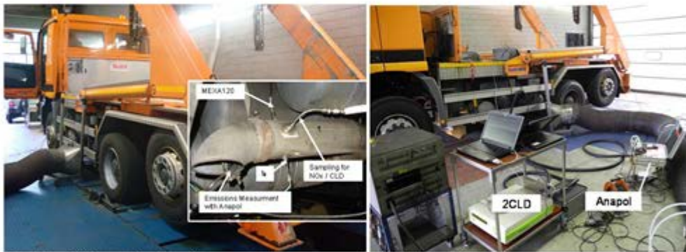
Tested vehicle and measuring apparatus on the LARAG HD chassis dyno
