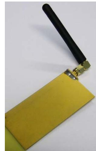
Antenna stubs attached to a small board
