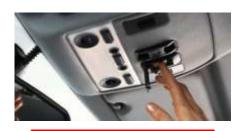
HMI conformity ✓ ECE121 Vehicles of category M1 and N1 not in the scope of UN R94 and/or R95 have to be equipped (at the minimum) with a manual activation of an emergency call.
