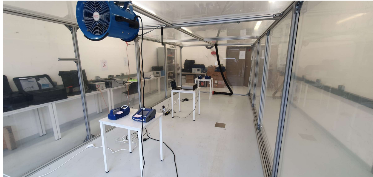
Fig 1: Closed chamber (measurement bubble)
