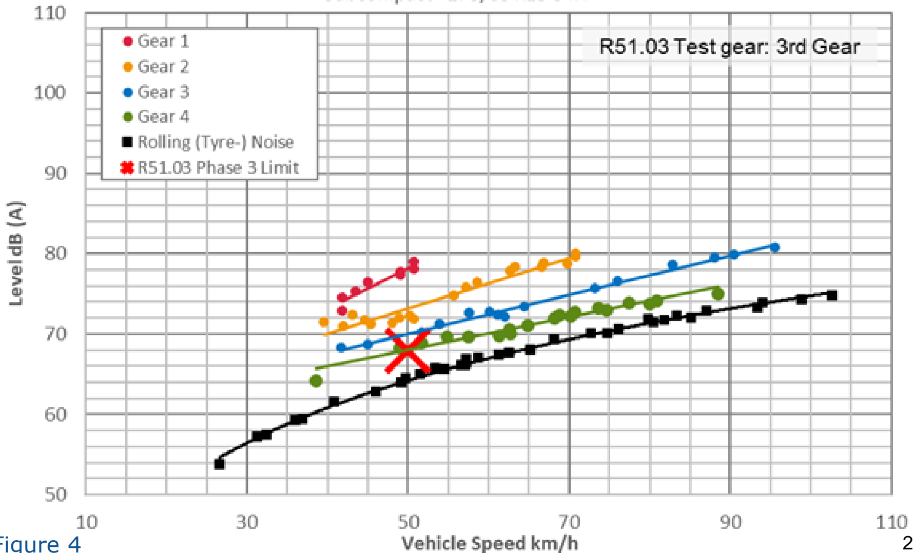
WOT Acceleration Noise & Tyre Rolling Noise Subcompact - 175/65 R15 84H
