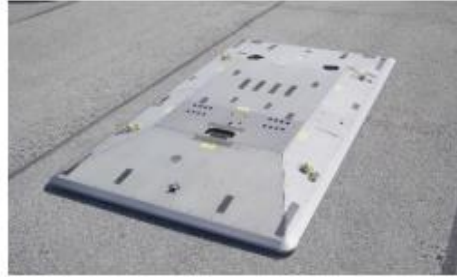
Guided Soft Target- M1 category vehicle soft target with motion platform
