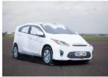
Guided Soft Target- M1 category vehicle soft target with motion platform
