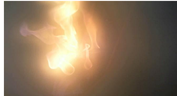
The Thermal runaway phenomenon of NMC Li-ion battery with 100 % SOC
