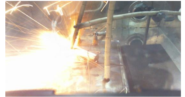
The Thermal runaway phenomenon of LCO Li-ion battery with 100 % SOC
