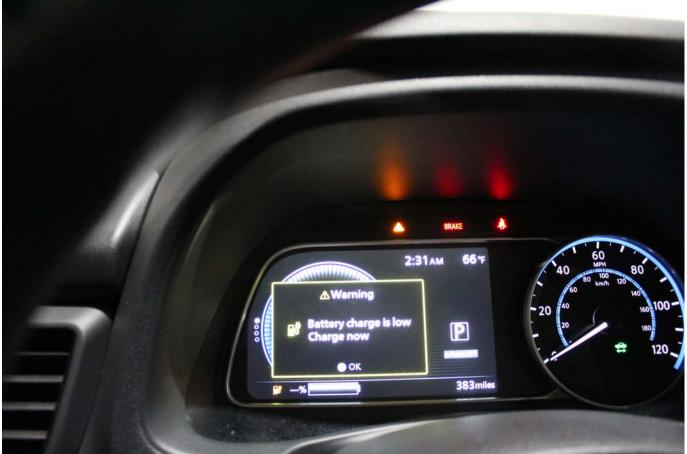
Photo No. 022 - Over-discharge Vehicle - Post Test
