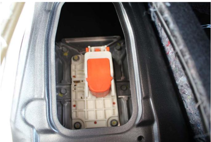
Photo No. 008 - Vehicle Manual Safety Disconnect Installed in Vehicle
