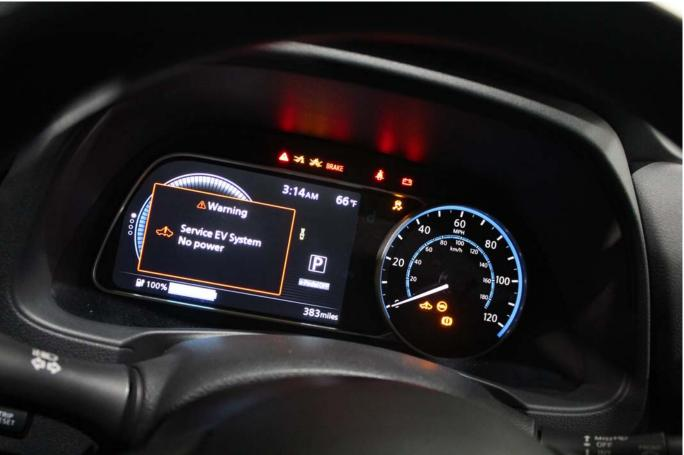
Photo No. 019 - Overcharge Vehicle - Post Test
