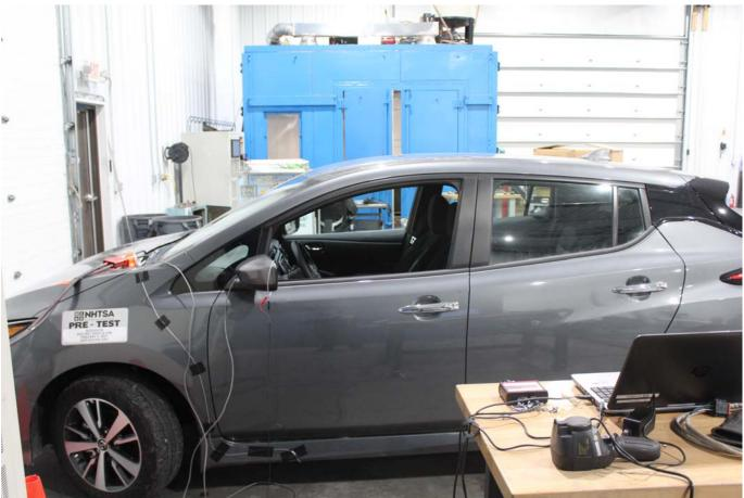
Photo No. 018 - Overcharge Test Setup
