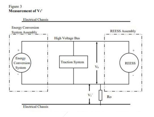
5. Calculate the electrical isolation (Ri) according to the following formula:  $Ri = Ro^*(V_b/V_1' - V_b/V_1)$  or  $Ri = Ro^*V_b^*(1/V_1' - 1/V_1)$  6. If V2 is greater than or equal to V1, a standard known resistance (Ro) is inserted between the positive side of the high voltage bus and the electrical chassis. With Ro installed, measure the voltage (V2') between the positive side of the high voltage bus and the electrical chassis (see Figure 4).
