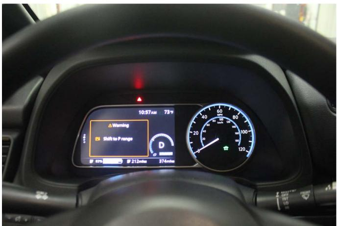
Photo No. 011 - Driver Leaving the Vehicle Indication
