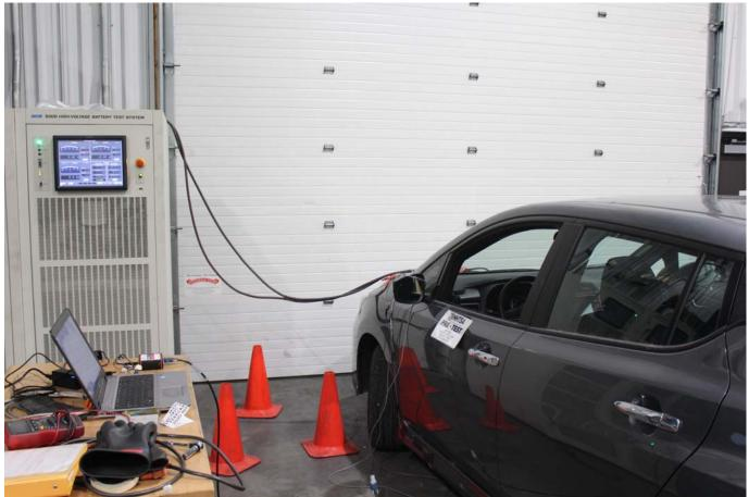
Photo No. 021 - Over-discharge Test Setup
