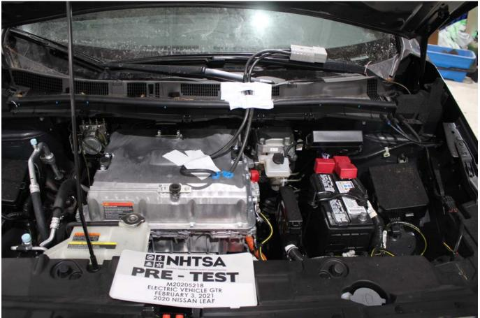
Photo No. 017 - Overcharge Breakout Harness
