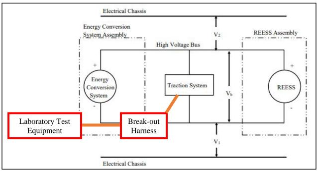
Figure 2- In-use Break-out Harness Test Setup
