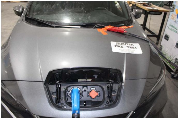
Photo No. 027 - Overcurrent Test Setup
