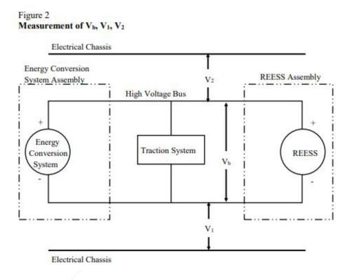
3. Measure and record the voltage (V1) between the negative side of the high voltage bus and the electrical chassis and voltage (V2) between the positive side of the high voltage bus and the electrical chassis (see Figure 2).
