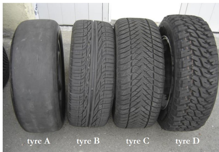
Figure 7-1: The four measurement tyres: A- Pirelli slick tyre, B- Pirelli summer tyre, C- Goodyear Eagle Ultra Grip winter tyre, D-Goodyear Wrangler 4x4 off-road tyre.
