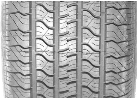
Figure 3 – The reference tyre (SRTT 16"); showing its tread pattern
