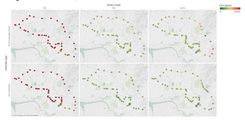
☑ In the AUTO mode, the RC mode was operated before the tunnel section, and the CO<sub>2</sub> conc. increased
