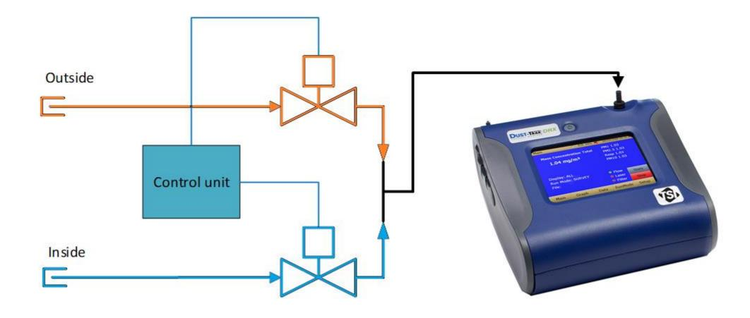
The length of sampling tubes for Outside and Inside channels are equal All tubes are made of antistatic plastics
