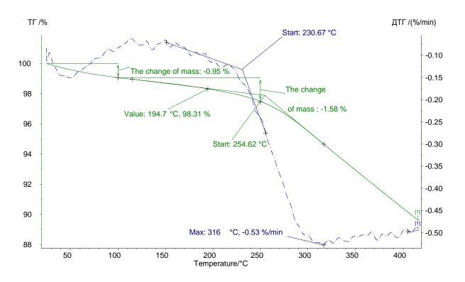
Picture 1– Fragment of the weight loss curve and its derivative for the mixture powders of asphalt pavement and used tires Nokia Rollster TS (the dimension 185/70 R14, manufacture - Finland)
