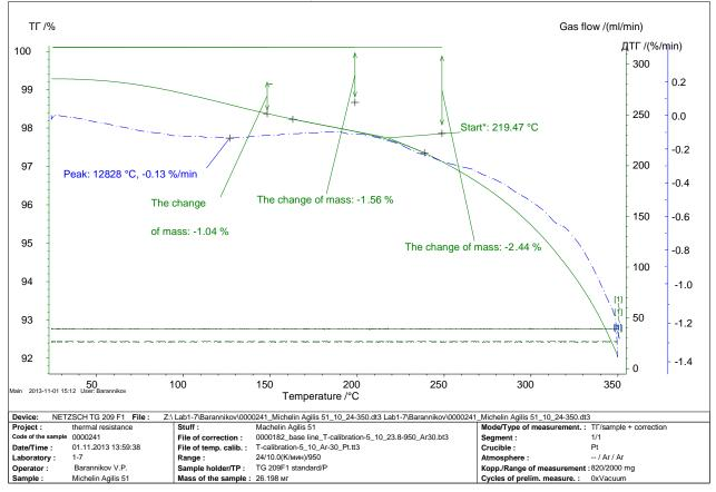
Picture 2 – Fragment of the weight loss curve and its derivative for the new tires Michelin Agilis 51 (the dimension 175/65 R14, manufacture - United Kingdom)
