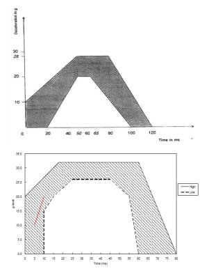
Draft AECS UN Regulation, Annex 7 requires to withstand acceleration of 75g for 1 to 5 ms → Level of acceleration is more representative of severe crash! Exceedance is very short (min. 1 ms); longer exceedance (e.g. 5 ms) would be more representative and still technically feasible.
