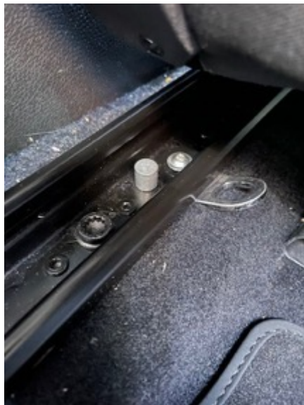
Retrofit lower tether anchorages
