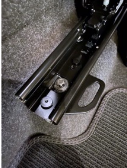
Integrated lower tether anchorages
