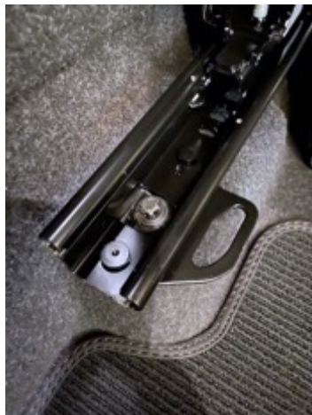
Integrated lower tether anchorages
