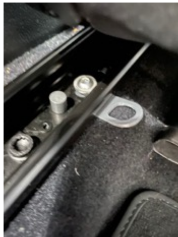
Retrofit lower tether anchorages
