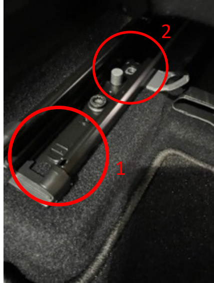
Retrofit lower tether anchorages
