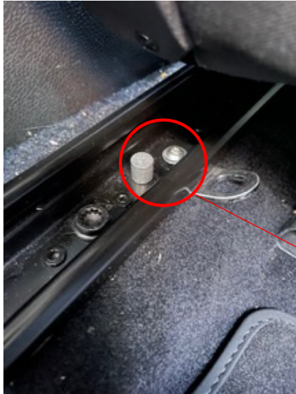
Retrofit lower tether anchorages
