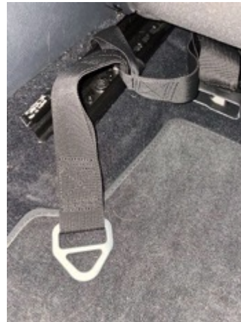
Lower tether anchor straps
