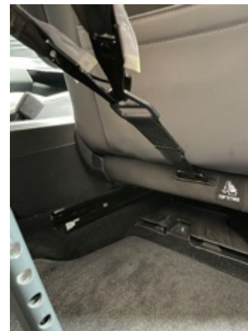
Top tether anchorage point
