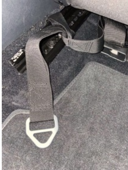
Lower tether anchor straps
