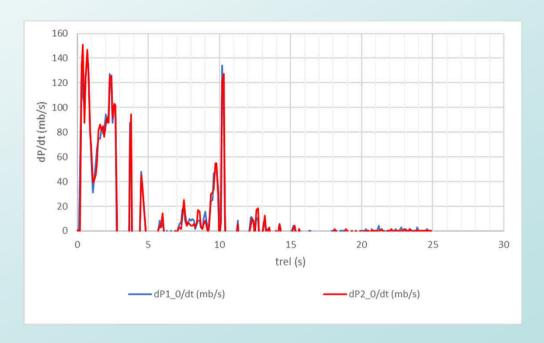
A lot of thin peaks. So dPpack/dt > 0.01 bar/s for at least 1s vs 3s to reduce false detection?
