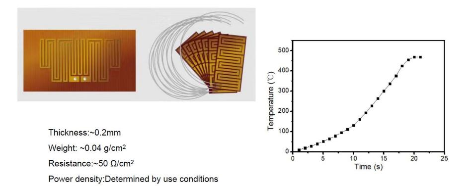
Surface area: ca. 70 cm<sup>2</sup>, adjustable Heating power: 500W constant power heating program (7.1 W/cm<sup>2</sup>)
