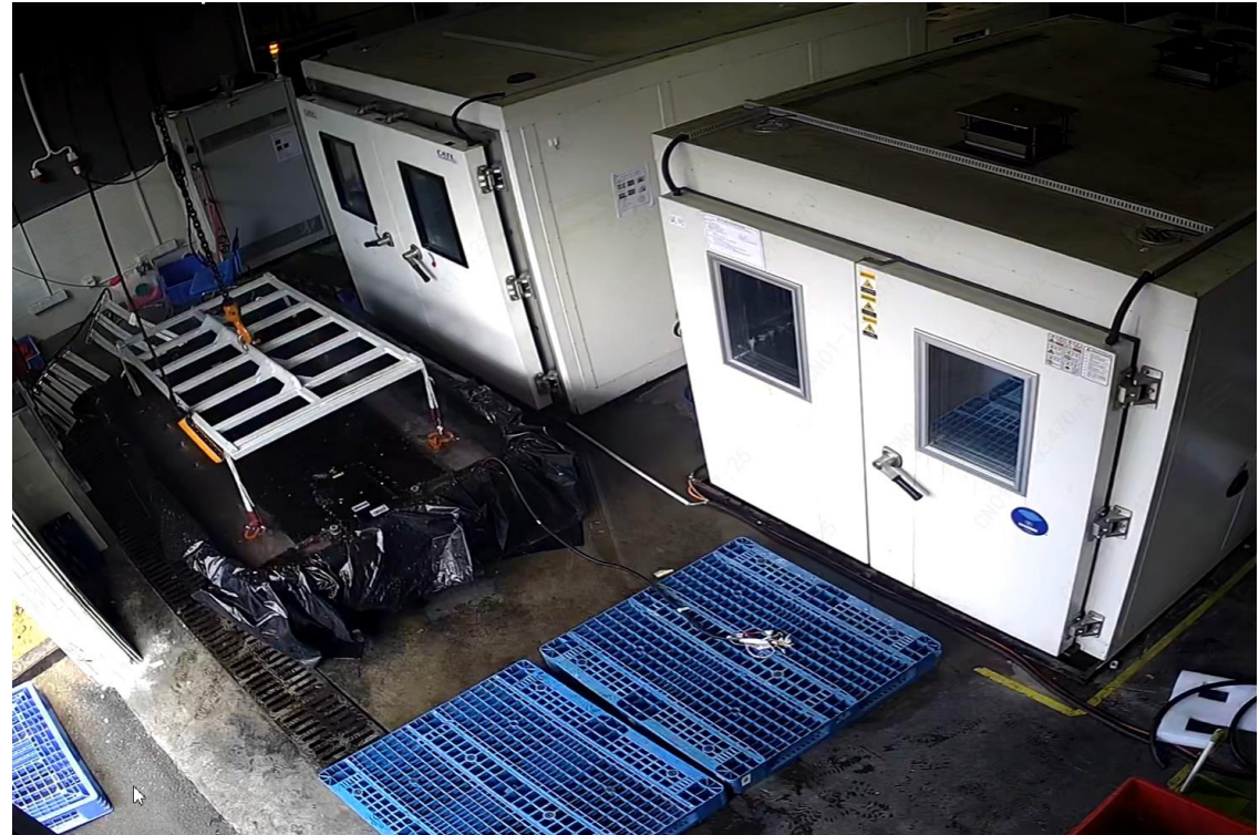
After battery pack immersed in salty water(3.5%) for 30mins , battery catch fire during lifting up from water tank.
