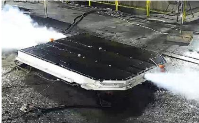
Cell thermal runaway (Degassing)
