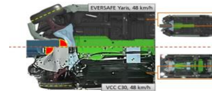
damage verification by component level
