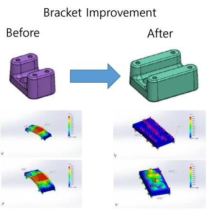
Simulation results with reduced Zaxis displacement at intermediate position and reduced area of stress damage in frame body
