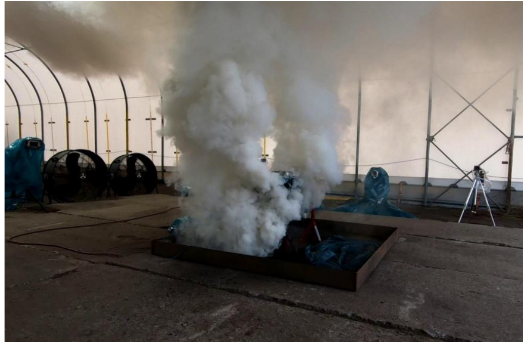
Test for qualification of a box for transport of critically defective LiBs, BAM TTS
