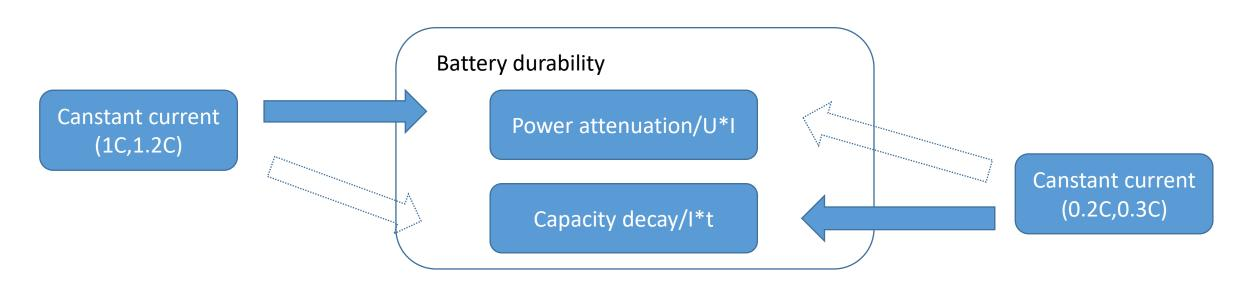
If we choose the canstant high current, the terminal for the old battery UBE test is result from the Power attenuation, we can't verify the capacity decay of in-vehicle battery.
