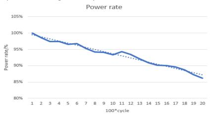
**Power attenuation**: the discharge power capacity decreases with the increase of the frequency of charging/discharging cycle.
