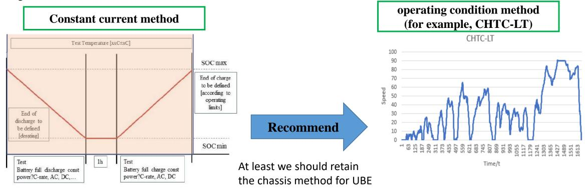
Constant current method: equivalent to the equal speed method, the discharge power/current value is constant. However, the vehicle cannot always travel at a uniform speed.
