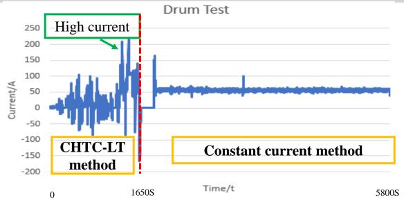
Comparison of test current value for 4.5t electric light truck CHTC-LT method and 70km/h vehicle speed (constant current method)
