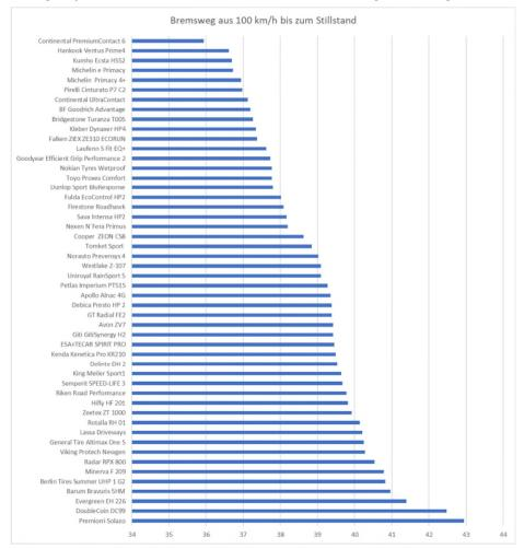
Diagram 1: Braking distances on dry asphalt
