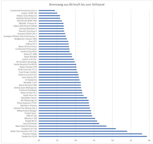
Diagram 1: Braking distances on wet asphalt
