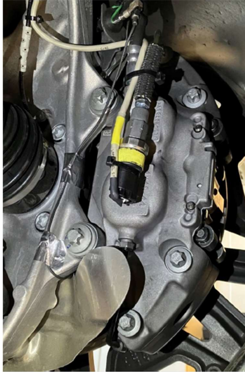
Figure 6.2. Brake pressure sensor at brake vent screw
