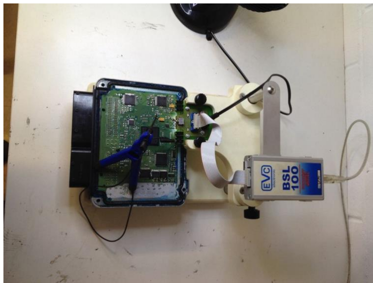
Figure 10. A BSL testbed [44]
