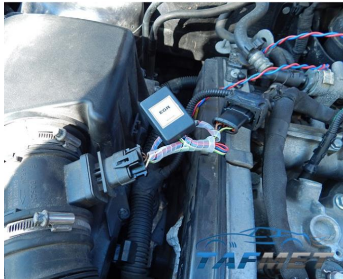
Figure 19. An EGR pneumatic valve emulator [41]
