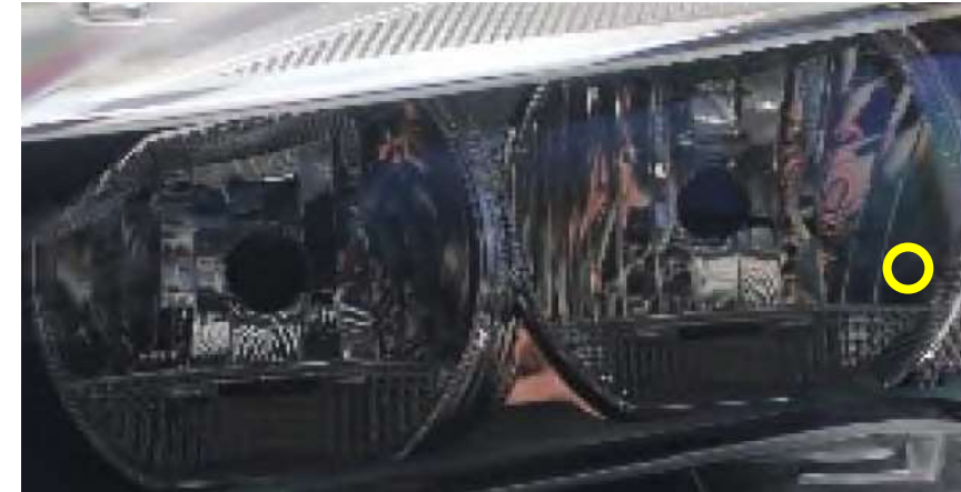
reflector and pin hole position creating filament image on the wall (10 m)
