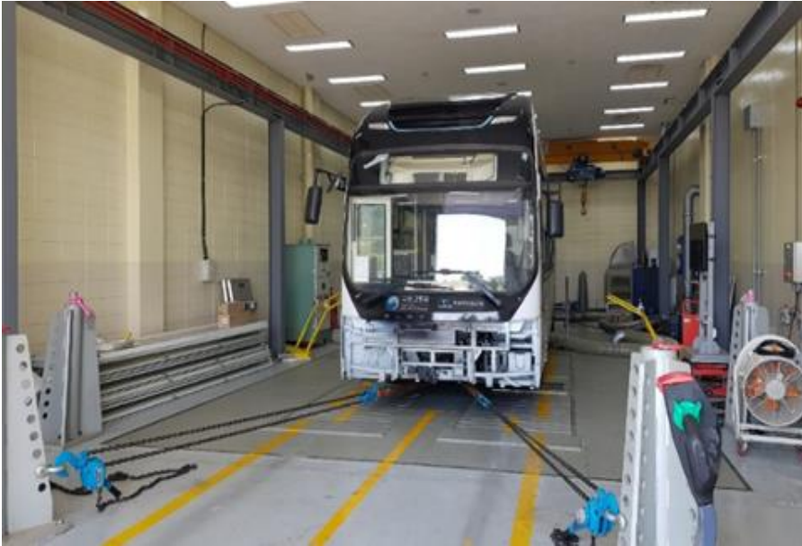
<Vehicle chassis dynamometer test>
