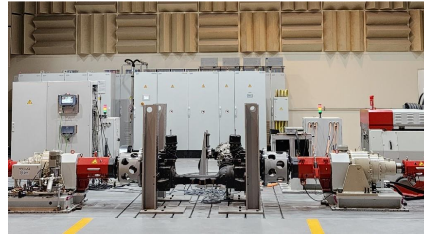
<Motor/Drive train bench hub dynamometer test>
