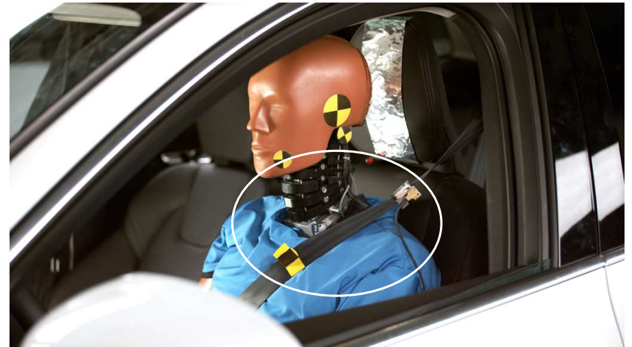
Volvo production reversible pretensioning activated prior to rear impact crash
