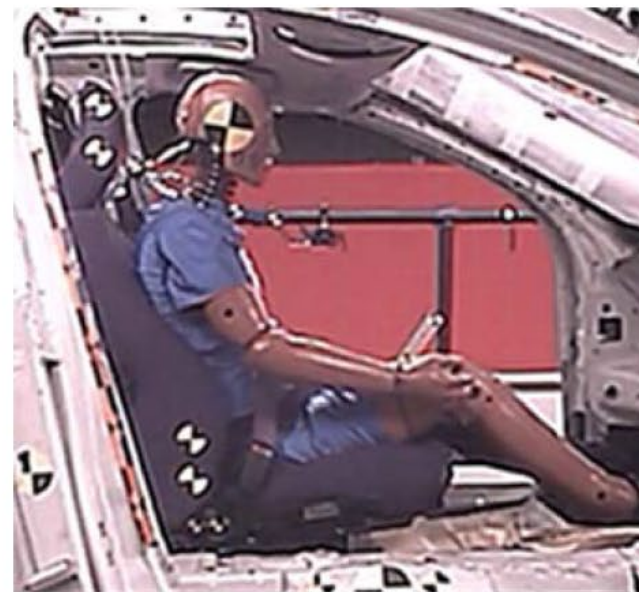
Fig. 3b. Occupant position after activation of electrical reversible pretension.
