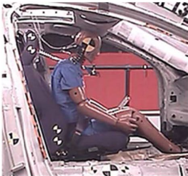
Fig. 3a. Initial occupant position at start of test.
