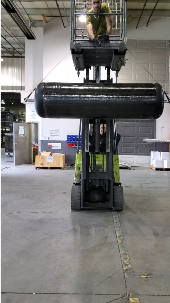
Type 4 drop test - If a cylinder is dropped, everyone will know it has happened
