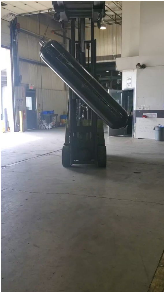
Type 3 drop test - If a cylinder is dropped, everyone will know it has happened
