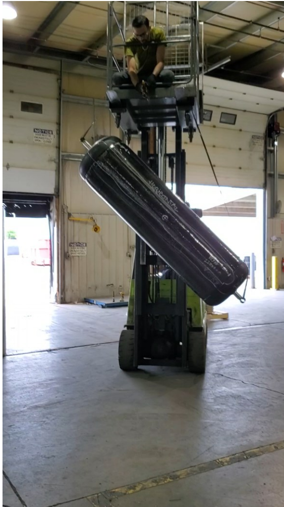
Type 4 drop test - If a cylinder is dropped, everyone will know it has happened
