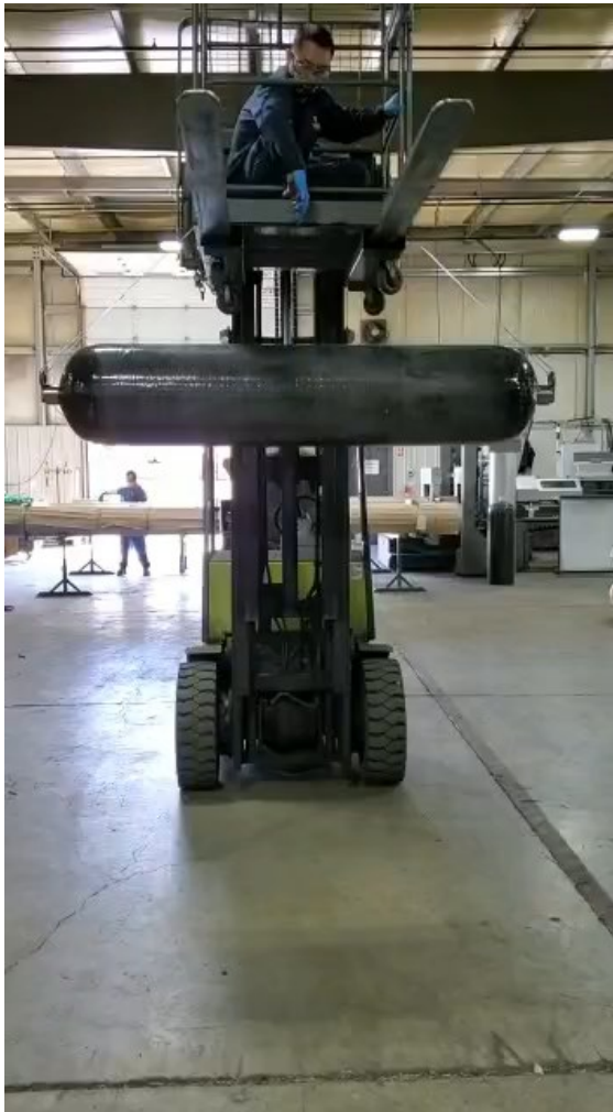
Type 3 drop test - If a cylinder is dropped, everyone will know it has happened
