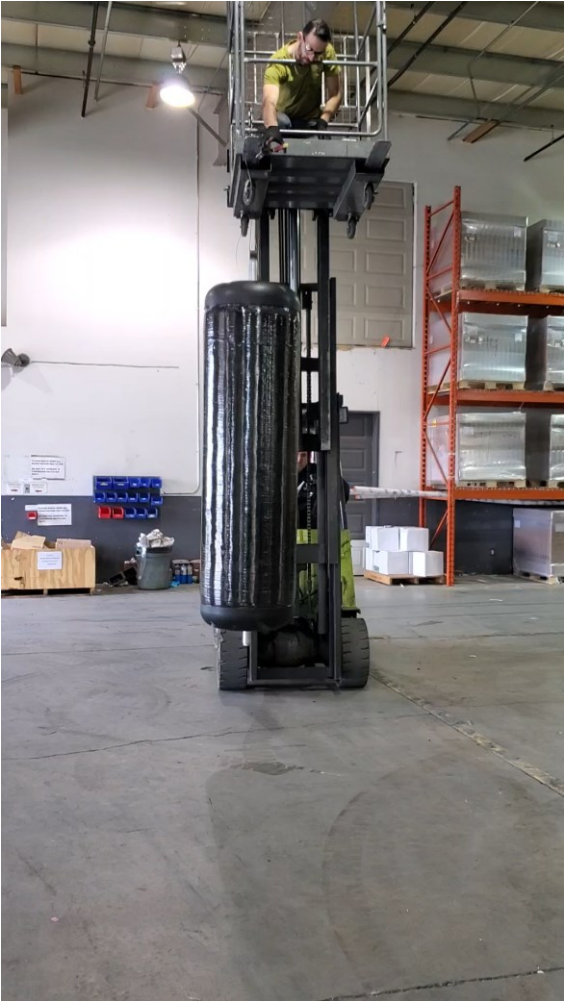
Type 4 drop test - If a cylinder is dropped, everyone will know it has happened
