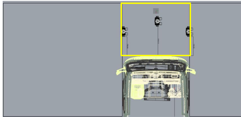
Plan view of the area within which the VRUs are contained, therefore VRU distance should correlate well with volume as per the previous uses of this method
