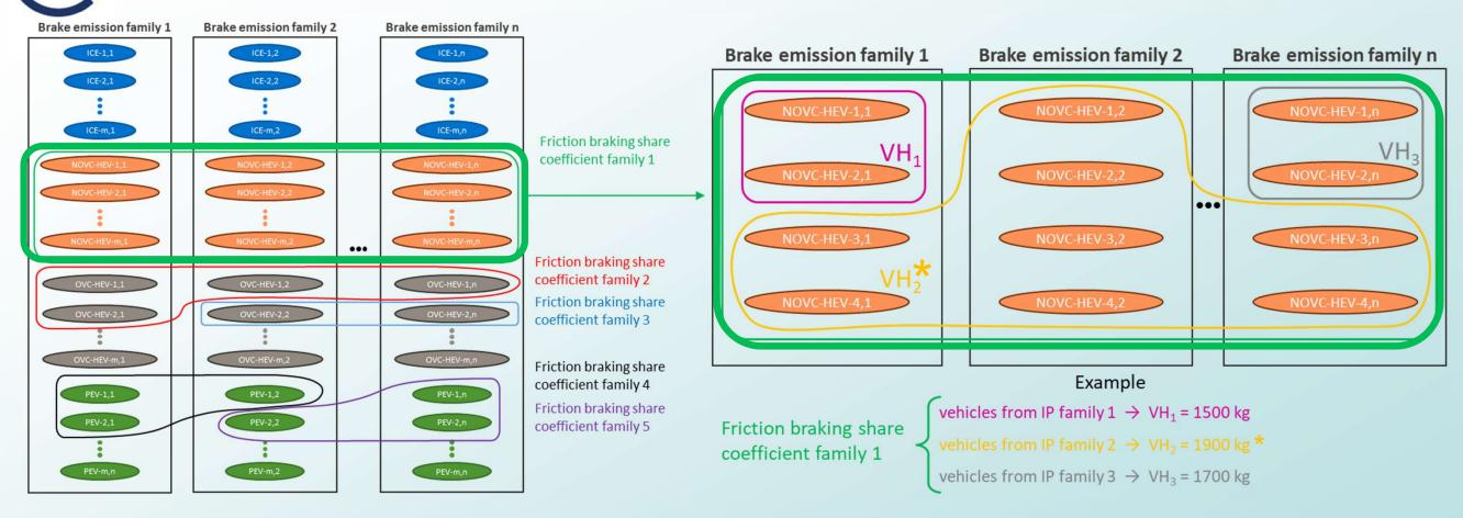
The Vehicle High with the highest test mass of a friction braking share coefficient family shall be selected for testing  $(VH_2^*)$  in the above example).
