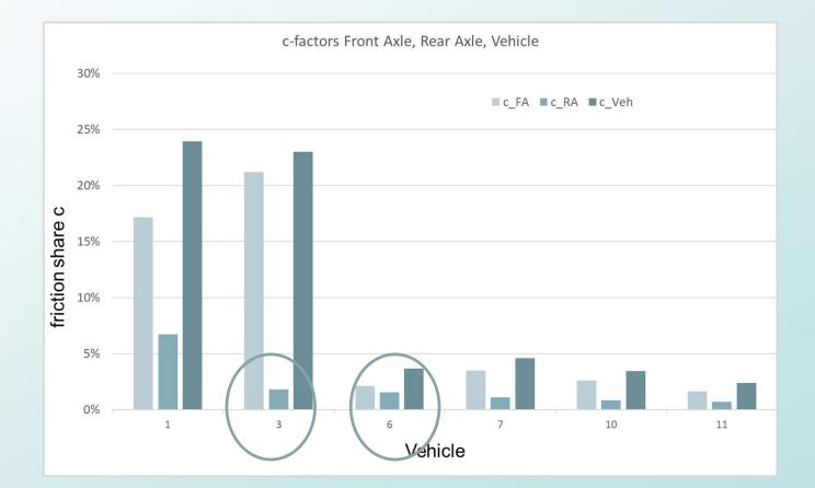
Depending on the front and rear axle brake emissions, this might impact vehicle brake emission.
