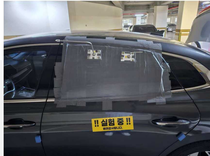
The outdoor air inlet and vent line
