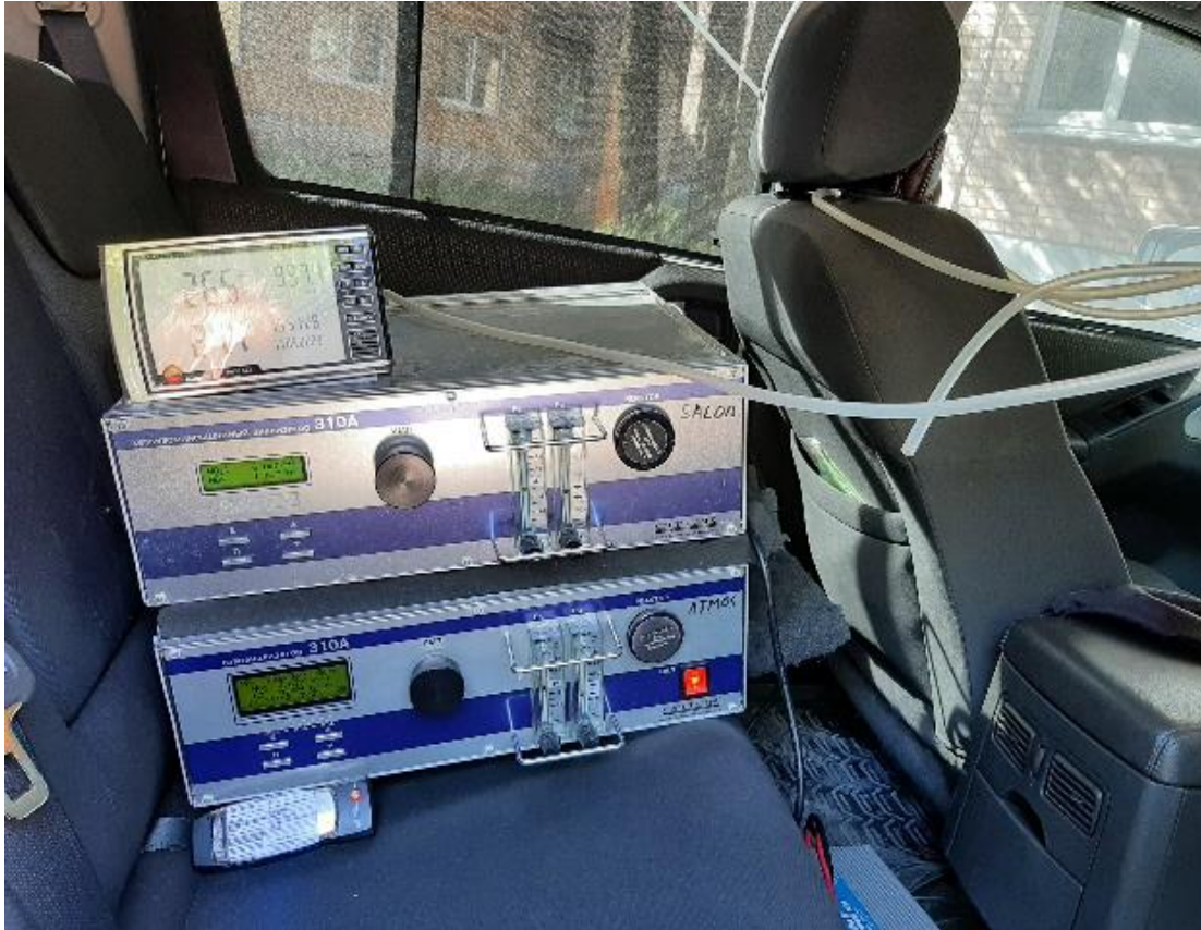
Two gas analyzers R-310 with chemiluminescent detector for measuring NO and NO2 Location in the cabin of tested car
