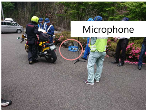
Street inspection : Stationary noise test
