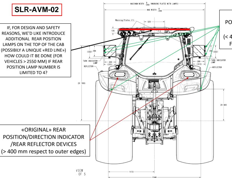
«ADDITIONAL» REAR POSITION/DIRECTION INDICATOR /REAR REFLECTOR DEVICES (< 400 mm respect to outer edges) For tractors width > 2550 mm
