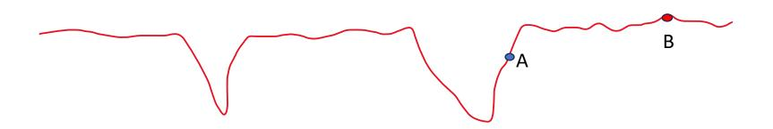
Take this as an example of a 1/3 octave vs. time. What do humans experience? We experience the peak levels, not the valleys. The 5-microphone array and max hold signal processing are designed to replicate this human perception. This is the same as how intermittent sounds are treated today (ISO, SAE, ECE, and FMVSS).
